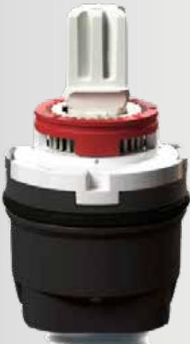
The EX-28 cartridge provides a slim design capability resulting in an interesting intermediate way between 35 mm and 25 mm taps. It features soft operational movement thanks to high grade ceramics and allows to aim for the most demanding standards, like NF-077 ECAU and low noise levels.
