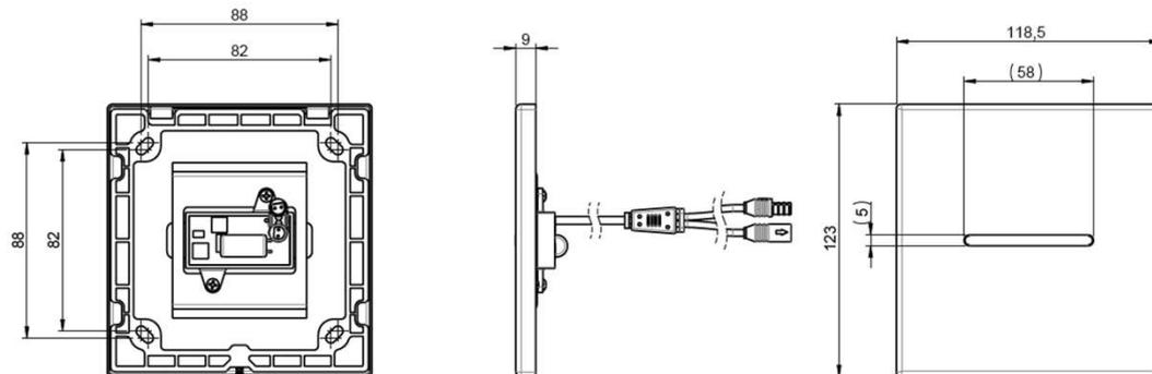
Tightening screws M4: 1,0-1,5 Nm
